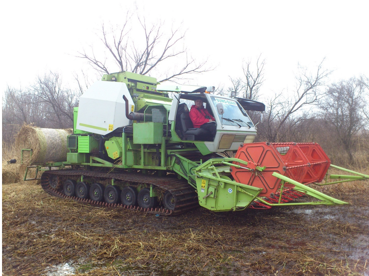
Figure 3: “Sumo-Quaxi” harvester for fully grown reed harvesting, during the harvesting operation in March 2012
