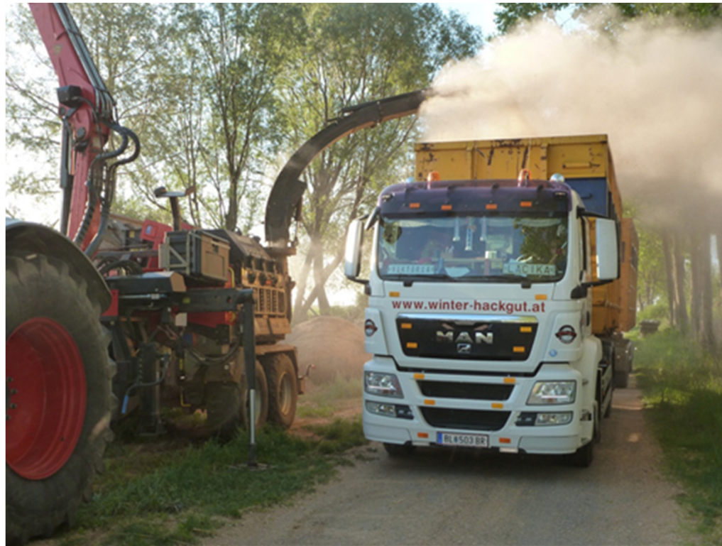
Figure 7: The chipper, driven by a tractor via a transmission shaft, fills the top-open container of the truck; considerable development of dust (May 2012)
