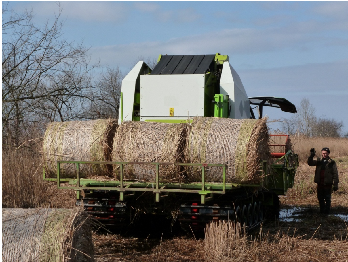
Figure 4: “Sumo-Quaxi” has reached the discharging place, 3 bales are dumped, the 4th bale is still in the bale press
