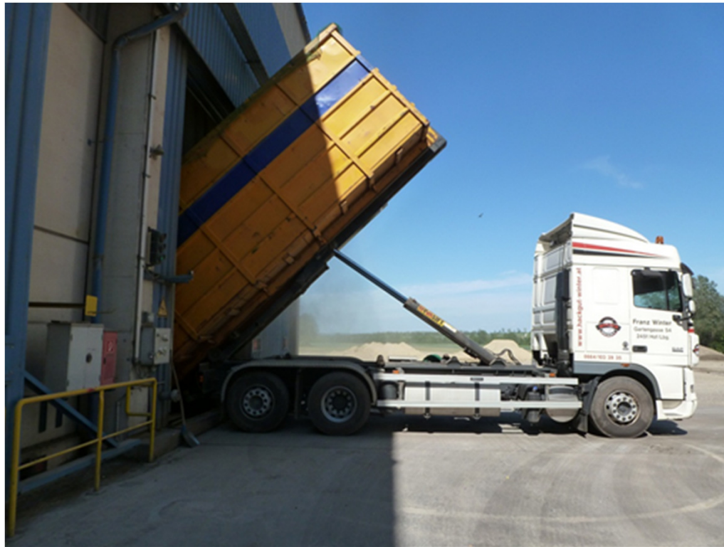
Figure 8: Skipping and discharging the chipped reed at the storage bin of the cement factory
